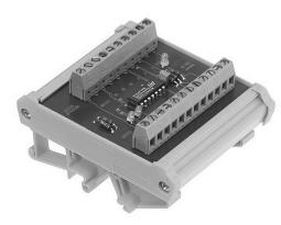
This interface module generates two additional static rotation direction signals (V, R) from the two output signals A, B phase-shifted by 90° of an incremental encoder.
